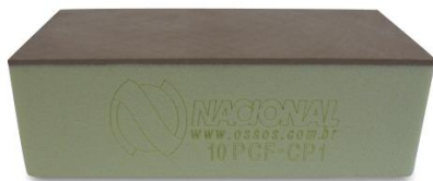
10PCF-CP1 - Block for biomechanical tests 10 pcf with 1 mm cortical W 4,5 X L 9,5 X H 3,1 CM
