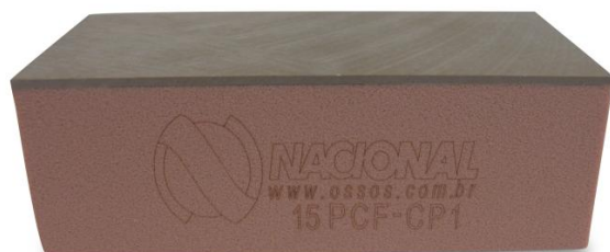
15PCF-CP1 - Block for biomechanical tests 15 pcf with 1 mm cortical W 4,5 X L 9,5 X H 3,1 CM
